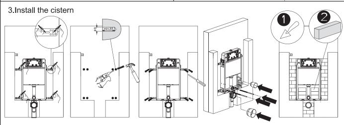
NOTE: the size unit is mm,  $\frac{9}{2}$  = the floor height after the project. The fill water pressure and stop filling pressure is between 0.01MPa-2.0MPa, water temperature: 2°C-45°C, flush volume can be adjustable.
